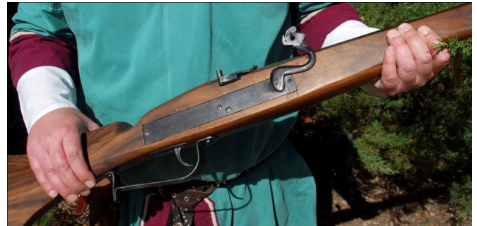
The lock and trigger mechanism of the arquebus. Note the s-shaped serpentine or “dog” and firing pan cover at the upper centre of the picture. The flat metal plate on the side of the weapon hides a simple spring and trigger-release mechanism.
