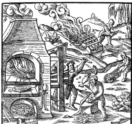
A—WOOD. B—BRICKS. C—PANS. D—FURNACE. E—CRUCIBLE. F—PIPE. G—DIPPING-POT.
